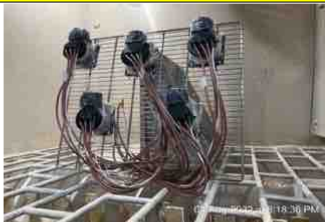
Fatigue test in Dusty environment
